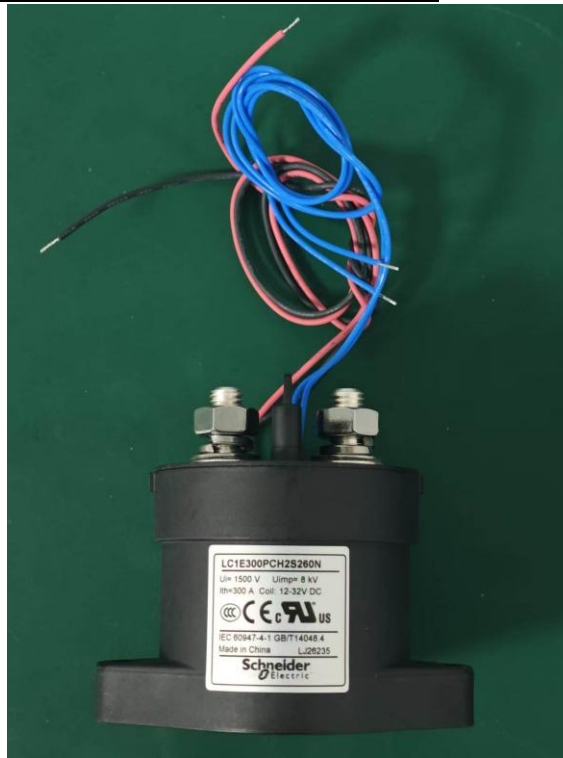
Figure 79 DC contactor KM1-KM4
