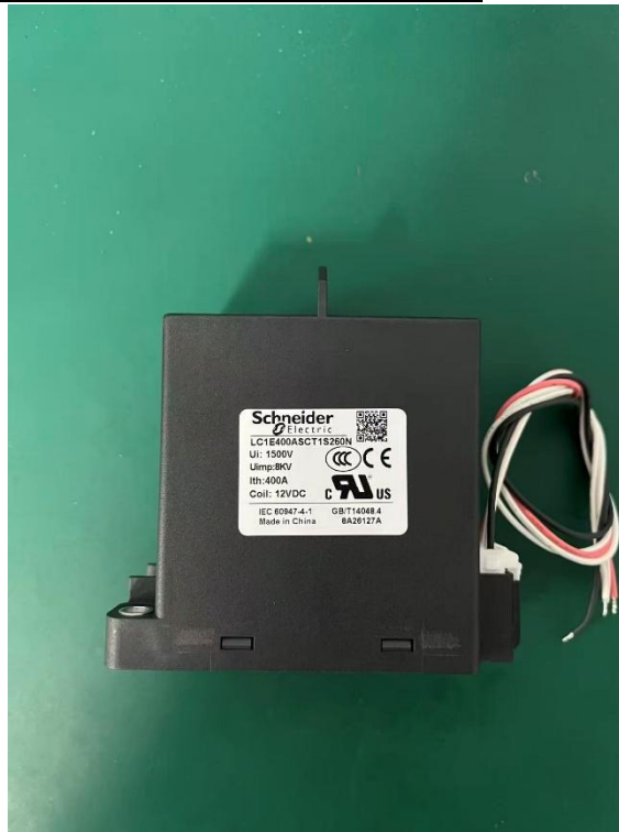
Figure 33 DC contactor KM1-KM4
