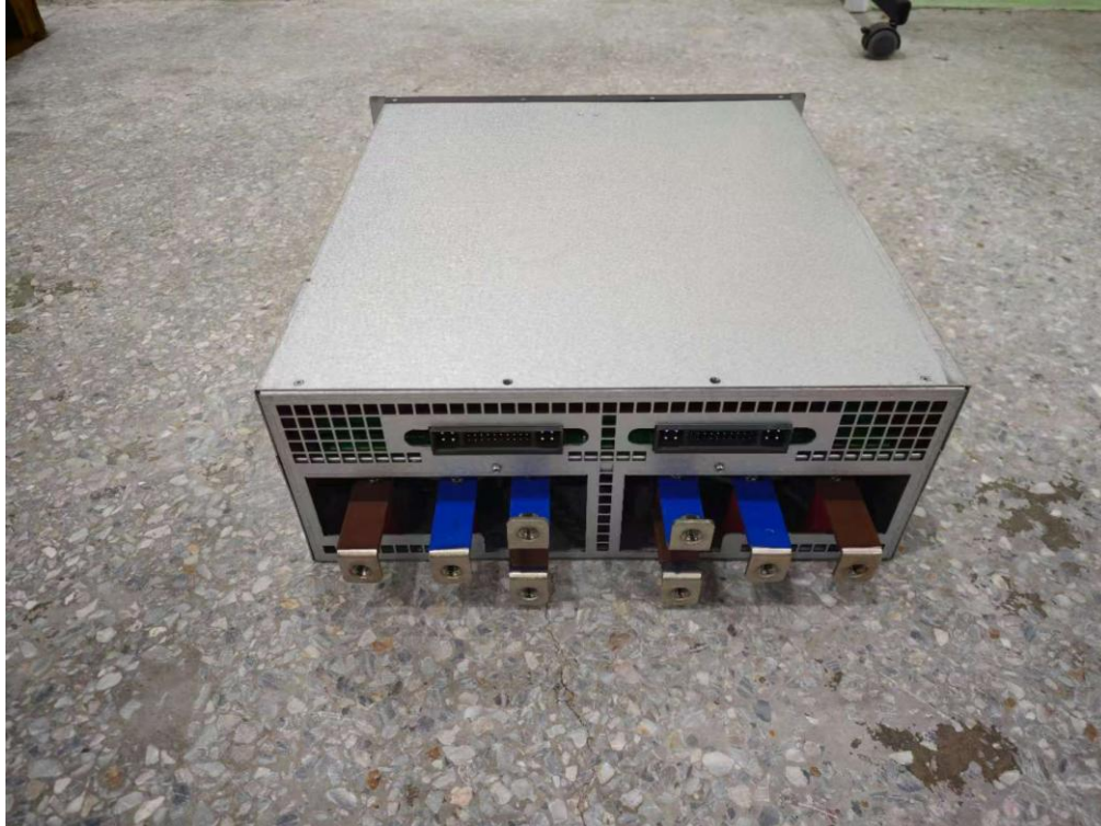
Figure 75 Rear of DC integrated module
