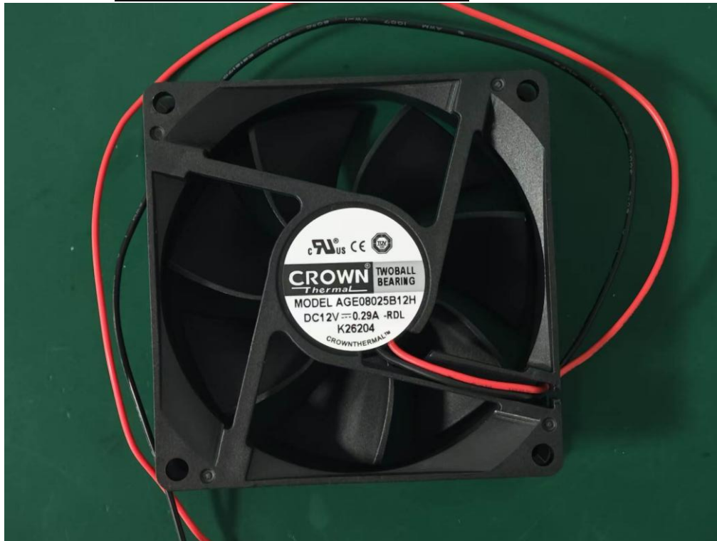
Figure 81 Marking plate of fan inside the DC integrated module
