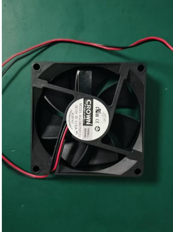
Figure 35 Marking plate of fan inside the DC integrated module
