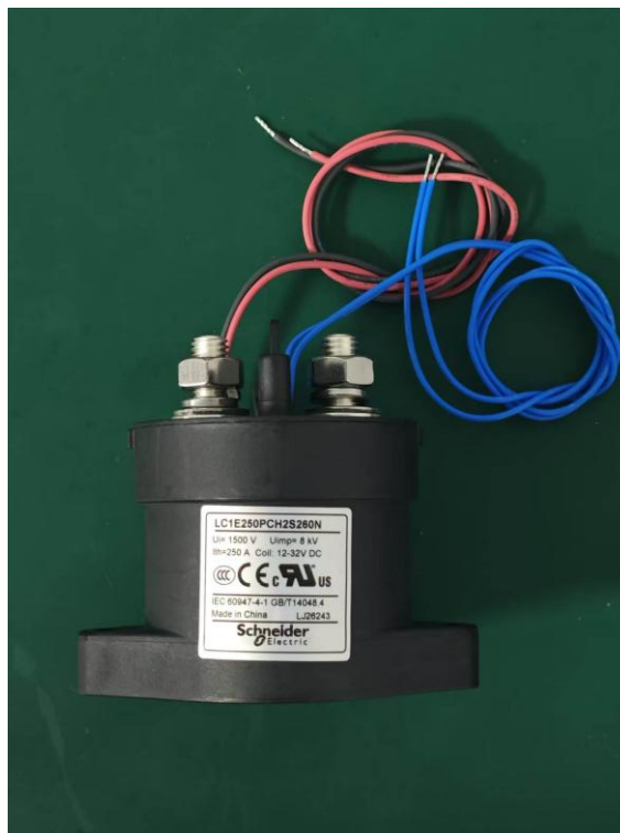
Figure 80 DC contactor KM5, KM6
