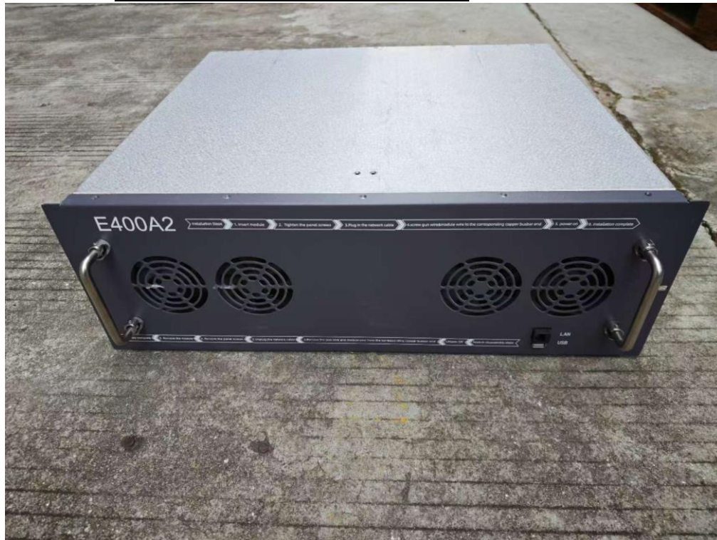
Figure 27 Front of DC integrated module
