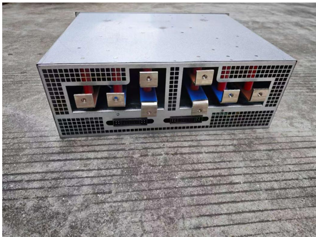
Figure 28 Rear of DC integrated module
